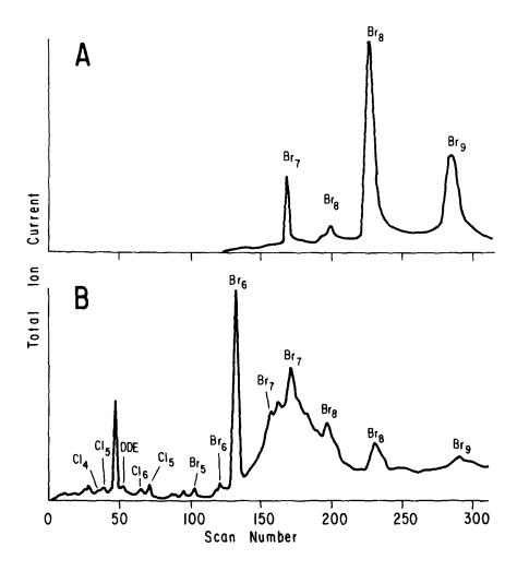
Fig. 1. Reconstructed gas chromatograms of OB (A) and extract of fish fed OB-contaminated food (B).
